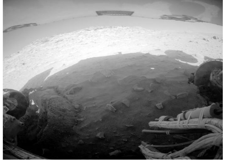
Spirit's view of its own predicament. The rover is now parked for the winter with its solar panels tilted only 9 degrees toward the sun. Spirit recorded this fisheye view with its rear hazard-avoidance camera after completing a drive during the 2,169th Martian day, or sol, of Spirit's mission on Mars (Feb. 8, 2010). The drive motor for the right-rear wheel (on the left in this view) stopped working in late 2009, leaving the six-wheeled rover with only four functioning wheels. The top of the image shows the underside of Spirit's solar array. Image Credit: NASA/JPL-Caltech
